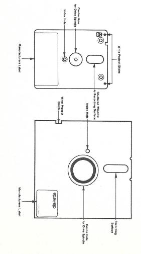
The write protection notch (or slide) shown in the diagrams enables the disc to be 'write protected'. When protected in this way (see Appendix 1) the disc cannot be written to, thus protecting the contents.
