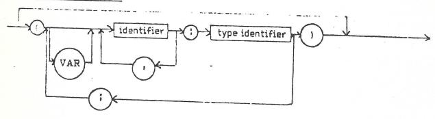
A type identifier must be used following the colon - otherwise \*ERROR\* 44 will result.
