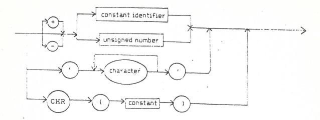
The non-standard CHR construct is provided here so that constants may be used for control characters. In this case the constant in parentheses must be of type integer.
