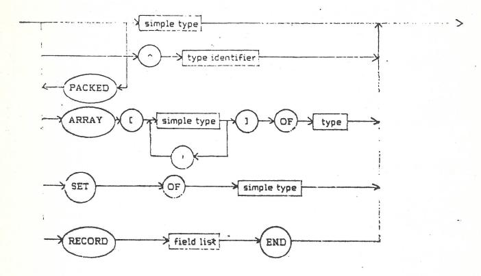
The reserved word PACKED is accepted but ignored since packing already takes place for arrays of characters etc. The only case in which the packing of arrays would be advantageous is with an array of Booleans – but this is more naturally expressed as a set when packing is required.
